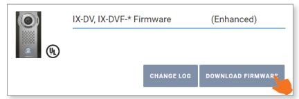
The firmware would usually be updated through IXG Support Tool, which is shown on the next page. For IX Series stations with a starting firmware version below 5.0, use the Aiphone IX Firmware Upgrade Tool instead. IXG Series stations have a different firmware numbering scheme and do not use this tool.
